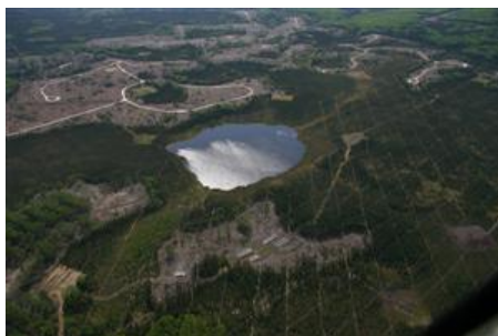
Seismic lines are cut across leases to map deep oil sands deposits. Source: David Dodge. Copyright © 2005 The Pembina Institute. www.oilsandswatch.org ( click to enlarge )
